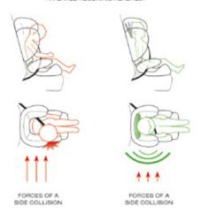
the child's head can remain within the safety zone of the seat. The patented head protection ensures a more comfortable sleeping position and enhanced safety compared to conventional systems.
